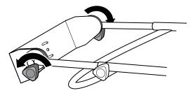
**2.** Loosen the adjustment knobs on each side of the foot plate.
