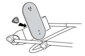
**4.** Reattach the foot plate to the foot plate bracket. Adjust for plantar/dorsiflexion and internal/external rotation as needed.
