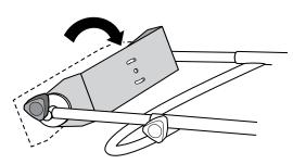
**3.** Rotate the foot plate bracket inward 180° as shown.
